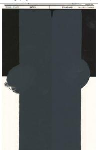
Solvent based Alkyd paint mixed with a universal colorant, No colour development of the bleu colorant. Adding 1% ADD-6215 post addition to the base paint showed clear improvement. (right side of draw down)
