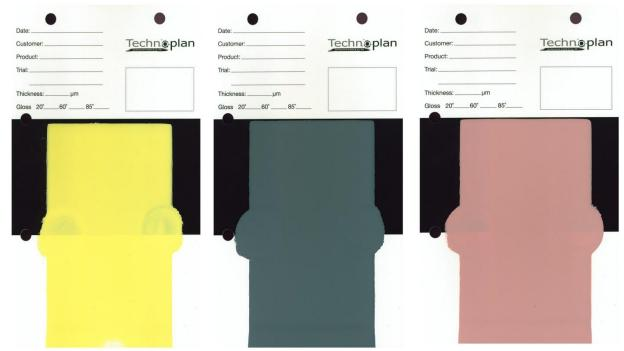
(80% transparent alkyd paint adding 18 % TiO2 colorant & 2% Yellow or Black or Red Iron oxide colorant all based on **ADD-6245**. Formulations are mentioned in the table on p.2 marked in orange.)
